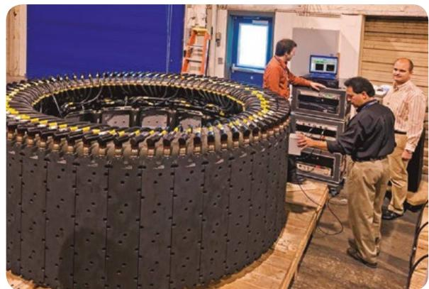
S-80 Plus bow mounted cylindrical array undergoing testing
